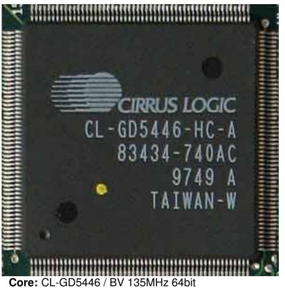
Core: CL-GD5446 / BV 135MHz 64bit Memory: 1-2MB (4MB max) EDO 80,538MHz 64bit Year: 1996 Bus: PCI Made: Taiwan Links: Pdf web archive Technical reference manual
