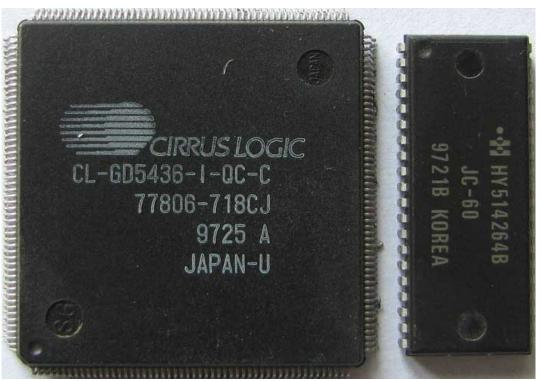
Core: CL-GD5436 ?MHz 64bit Memory: 1MB FPM (EDO) 50,11 (80 max) MHz 64bit Year: 1995 Bus: integrated, PCI Made: Japan, Korea Links: <u>Pdf</u> <u>Press</u>
