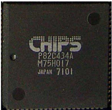
Core: P82C434A+P82C431 ?MHz ?bit Memory: 256kB ?MHz ?bit Year: 1985 Bus: ISA 8bit Made: Japan Links: <u>Pdf</u>
