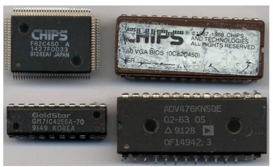
Core: F82C450 ?MHz ?bit Memory: 512kB ?MHz ?bit Year: 1988 Bus: ISA 16bit
