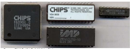
Core: F82C451C 36MHz ?bit Memory: 256kB ?MHz 8bit Year: 1990 Bus: ISA 16bit Made: USA, Japan Links: Pdf
