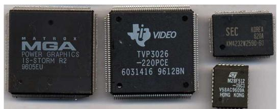
Core: IS STORM/MGA-2064W 50,113/59,99MHz 64bit Memory: 2/4MB(8MB max) WRAM 50,113/59,99MHz 64bit Year: 1995 Bus: PCI Made: NEC 0,35 μm Links: stason.org czech review infoworld Datasheet Price: \$326
