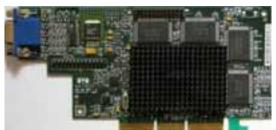
Core: MGA-G400 126MHz 256bit Memory: 16MB(32MB max) SGR 168MHz 128bit Year: 1999 Bus: AGP 4x Made: 0,25 μm Links: Wikipedia FiringSquad Datasheet Price: \$140
