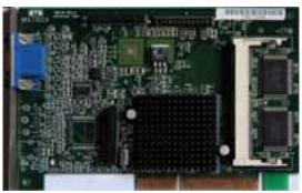
Core: MGA-G200 (Eclipse) 84,4MHz 128bit Memory: 8MB(16MB max) SGR 112,5MHz 64bit
