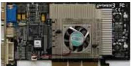
Core: NV20 200MHz 256bit Memory: 64MB DDR 458MHz 128bit Year: 2001 Bus: AGP 4x Made: TSMC 150nm Links: <u>iXBT Labs</u> <u>Techreport</u> <u>Wikipedia</u> Price: \$359
