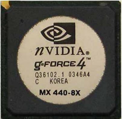
Core: NV18 250MHz (default is 270MHz) 256bit Memory: 64MB DDR 378MHz (default is 400MHz) 64bit Year: 2002 Bus: AGP 8x Made: TSMC 150nm Korea Links: <u>iXBT Labs</u> <u>Wikipedia</u> Price: \$145
