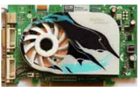
**Core:** G84 540MHz 32 shaders at 1188MHz **Memory:** 256MB GDDR3 1404MHz 128bit
