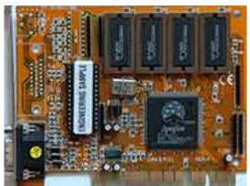
Core: OTI-64111 ?MHz 64bit Memory: 2MB (4MB? max) EDO ?MHz 64bit Year: 1995 Bus: PCI Made: ? Links: Press
