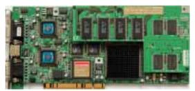
Core: 3DLabs GLiNT 500TX + GLINT Delta ?MHz ?bit + Avance Logic ALG2564 for DOS Memory: 8MB VRAM + 16MB EDO + 1MB for DOS ?MHz ?bit Year: 1996 Bus: PCI
