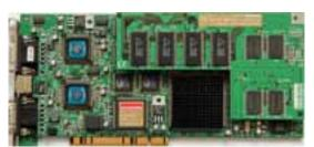
**Core:** 3DLabs GLINT 500TX + GLINT Delta ?MHz ?bit + Avance Logic ALG2564 for DOS **Memory:** 8MB VRAM + 16MB EDO + 1MB for DOS ?MHz ?bit **Year:** 1996 **Bus:** PCI **Made:** ? Links: Press drivers Opengl Price: \$2,795
