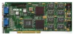
Core: 2x3Dlabs Permedia 2 80MHz 64bit
