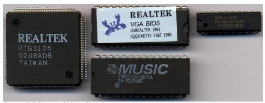
Core: RTG3106 ?MHz ?bit Memory: 512kB ?MHz ?bit Year: 1991 Bus: ISA 16bit
