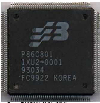
Core: P86C801 ?MHz 32bit Memory: 1MB FPM ?MHz ?bit Year: 1992 Bus: ISA 16bit Made: Korea Links: Gbooks
