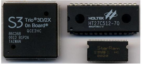
Core: 86C368 83/100MHz 128bit Memory: 4-8MB SGR/SDR 83/100MHz 64bit Year: 1999 Bus: AGP 2x Made: Taiwan, Korea Links: none known
