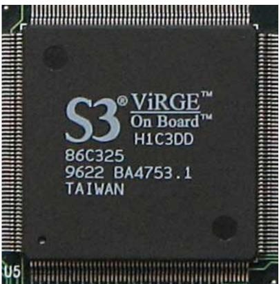
Core: 86C325 50,11/54,89MHz 64bit Memory: 2-4MB 1 cycle EDO 50,11/54,89MHz 64bit Year: 1995 Bus: PCI Made: Taiwan Links: Pdf Vintage3D Datasheet
