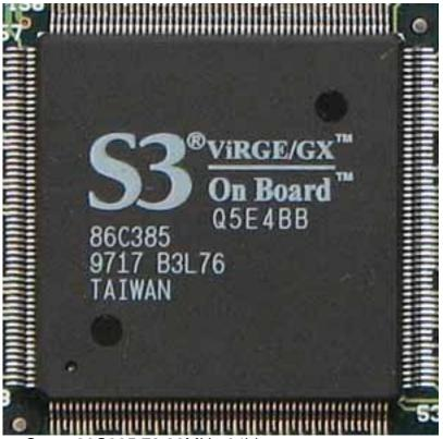
**Core:** 86C385 73,38MHz 64bit **Memory:** 4MB SGR 73,38MHz 64bit
