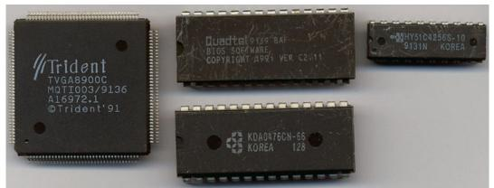
Core: TVGA 8900C ?MHz ?bit Memory: 1MB ?MHz ?bit Year: 1991 Bus: ISA 16bit Made: Korea, Japan Links: none known Gift from: Vegan
