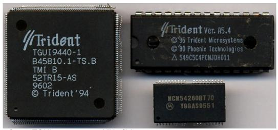
**Core:** TGUI 9440-1 57,27MHz ?bit **Memory:** 1MB (2MB max) 57,27MHz ?bit
