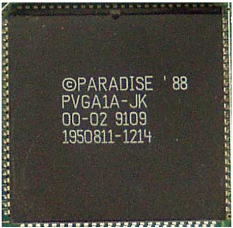
Core: PVGA1A-JK ?MHz ?bit Memory: 256kB ?MHz ?bit Year: 1988 Bus: ISA 8/16bit Made: ? Links: none known
