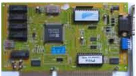
Core: WD90C11-LR 65MHz 16bit Memory: 512kB 42MHz 16bit Year: 1990 Bus: ISA 16bit Made: 1.25 μm Links: Datasheet
