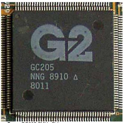
Core: GC205 ?MHz ?bit Memory: 256kB ?MHz ?bit Year: 1989 Bus: ISA 16bit Made: ?? Links: none known
