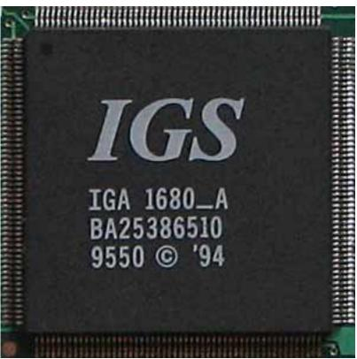
Core: IGA 1680\_A ?MHz ?bit Memory: 1MB 60MHz ?bit Year: 1994 Bus: PCI
