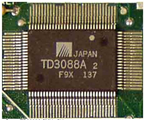
Core: TD3088A ?MHz ?bit Memory: 64kB ?MHz ?bit Year: 198 Bus: ISA 8bit Made: Japan Links: Jumpers
