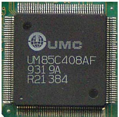
Core: UM85C408AF ?MHz ?bit Memory: 256kB (1MB max) ?MHz ?bit Year: 1993 Bus: ISA 16bit Made: UMC Links: none known
