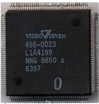
Core: L1A4199 ?MHz ?bit Memory: 256kB ?MHz ?bit Year: 1988 Bus: ISA 16bit
