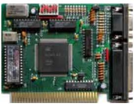
Core: D10 ?MHz ?bit Memory: 64kB ?MHz ?bit Year: 1985 Bus: ISA 8bit
