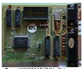
Core: W86855AF ?MHz ?bit Memory: 64kB ?MHz ?bit Year: 198? Bus: ISA 8bit Made: ? Links: none known
