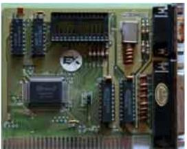
Core: W86855AF ?MHz ?bit Memory: 64kB ?MHz ?bit Year: 198? Bus: ISA 8bit Made: ? Links: none known
