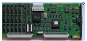
Core: Texas Instruments TMS34010FNL-50 50MHz 32bit
