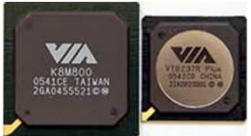
Graphic Core: S3 UniChrome Pro 200MHz 128bit Memory: 64MB DDR 400 / DDR2 667 64/128bit Year: 2004 CPU Socket: 754, 939, AM2 Made: Taiwan Links: <u>VIA</u> <u>VIApress</u> Note: from Gigabyte K8VM800M
