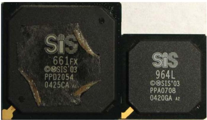
Graphic Core: SiS 315 200MHz 256bit Memory: 64MB DDR400 64bit Year: 2003 CPU Socket: 478 Made: SiS Links: <u>SiS</u> <u>Tom's Hardware</u>
