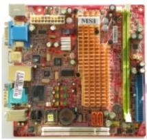
Core: VIA/S3 UniChrome IGP Pro 200MHz 128bit Memory: 64MB DDR2 533MHz 64bit
