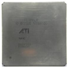
Core: Flipper 162MHz ?bit
