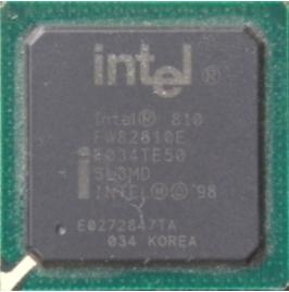
Core: Intel 82810E 100MHz Memory: 8MB SDR 133MHz 64bit Year: 1998 Bus: Integrated DirectX: 6.0 OpenGL: 1 ROPs: 1 TMUs: 1 CPU socket: 370
