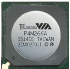
Core: S3 ProSavage8 ?MHz 128bit Memory: 64MB DDR400 64bit Year: 2001 Bus: Integrated CPU Socket: 478
