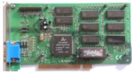
Core: ProMotion aT3D 50MHz 128bit Memory: 4MB EDO 50MHz 64bit Pixel pipelines:
