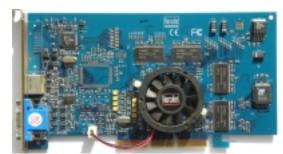
Core: STG4500-X 175MHz 128bit RAMDAC clock: 300MHz
