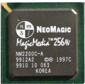
Core: Neomagic MagicMedia 256AV (NM2200C-A) ?MHz 256bit Memory: 1MB SDR 100MHz 64bit Year: 1997 Bus: Integrated AGP
