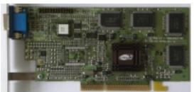
Core: ATI Rage 128GL 103MHz 128bit Memory: 16/32MB SGRAM/SDR 103MHz 128bit Year: 1998 Bus: AGP 2x Made: 250nm Vertex shaders: not supported Supported DirectX: 6.0
