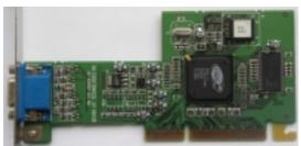
Core: ATI Rage XL 85MHz 64bit Memory: 8-16MB SDR 83,82MHz 64bit Year: 1999 Bus: AGP 2x Made: 350nm Vertex shaders: not supported supported DirectX:
