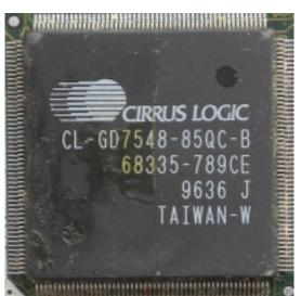
Core: CL-GD7548-85QC-B 80MHz 64-bit Memory: 1MB EDO 66MHz 64bit Year: 1995 Bus: Integrated PCI
