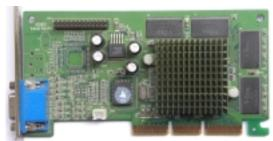
Core: NV11 175MHz 256bit Memory: 32MB SDR 166MHz 64bit Pixel pipelines: 2 TMU per pipeline: 2 Pixel shaders: 2 (v0.5) Vertex shaders: not supported
