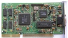
Core: TVGA 9000C ?MHz ?bit Memory: 512kB DRAM ?MHz ?bit Year: 1992 Bus: ISA 16bit Made: TSMC Taiwan
