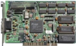
Core: TGUI9440 50MHz Memory: 2MB EDO 50MHz Year: 1994 Bus: PCI
