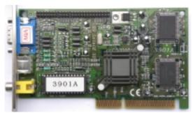
Core: 86C390 100MHz 128bit Memory: 8MB SGRAM 120MHz 64bit Year: 1998 Bus: AGP 2x I Made: 250nm Pixel Pipelines: 1 TMU per pipeline: 1
