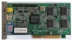
Core: 86C357 100MHz 64bit Memory: 4MB SGR 100MHz 64bit Year: 1997 Bus: AGP 1x Made: Philippines
