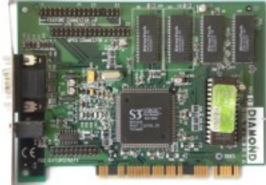
Core: 86c325 50MHz 64bit Memory: 2/4MB EDO 50MHz 64bit Year: 1995 Bus: PCI Pixel pipelines: 1 TMU per pipeline: 1 Pix
