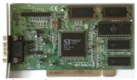
Core: 86C775 65MHz 64bit Memory: 2MB EDO 65MHz 64bit
